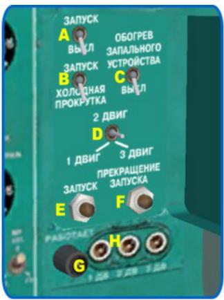
Fig. 12. Engine start panel
