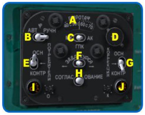
Fig. 5. PU-11 TKS compass system.
